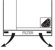
Locate access door marked "FILTER" and lift up the open side of the levers.
