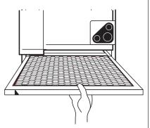
Slide dirty filter out, replace with a new filter making sure the arrows printed on it are pointing in the direction of airflow
